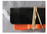
Step 2. Remove part of the label covering the ball as shown. Use a sharp knife to cut the label and then using same tool raise the corners of the label to peel it back. It is easiest if you have a pair of tweezers but is not absolutely necessary. Alternatively just remove a small part of the label above the ball. Easiest.
